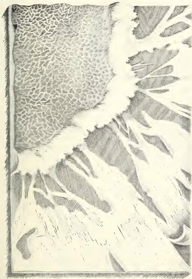
"DRY ROT," showing the fruiting portion ; also the white spreading felt-like mycelium.
